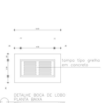
DETALHE BOCA DE LOBO PLANTA BAIXA ESCALA 1/100
