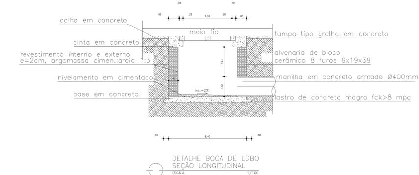
DETALHE BOCA DE LOBO SEÇÃO LONGITUDINAL ESCALA 1/100
