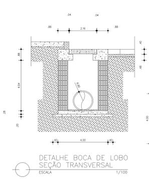
DETALHE BOCA DE LOBO SEÇÃO TRANSVERSAL ESCALA 1/100
